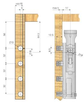
$<sup>^{\</sup>star}$  To achieve a nominal capacity of 65kg a Ø3.5x20 screw has to be screwed into the indicated fixing hole.
